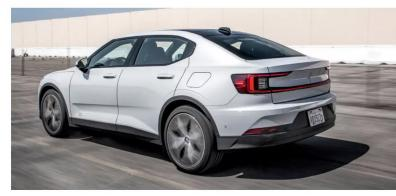
As of now, all Polestar 2s are equipped with front and rear motors with a total system output of 402 hp and 487 lb-ft of torque. Due to the permanent-magnet nature of the motors-meaning they must always be driven and can't freewheel—the Polestar 2's range pales in comparison to the rival Tesla Model 3, which nets 141 mpg-e combined and 250 miles of range on the EPA cycle to the Polestar's 92 mpg-e and 233 miles of range. And for 2021, Tesla is promising 263 miles of range on a base Model 3.
