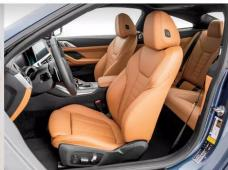
**VEHICLE LAYOUT** Front-engine, AWD, 4-pass, 2-door coupe **ENGINE/TRANSMISSION** 3.0L turbo DOHC 24-valve I-6/8-speed automatic **CURB WEIGHT (F/R DIST)** 3,960 lb (54/46%) **WHEELBASE** 112.2 in **LENGTH x WIDTH x HEIGHT** 188.0  $\times$  72.9  $\times$  54.8 in **ENERGY CONS, CITY/HWY** 153/112 kWh/100 miles **CO2 EMISSIONS, COMB** 0.78 lb/mile
